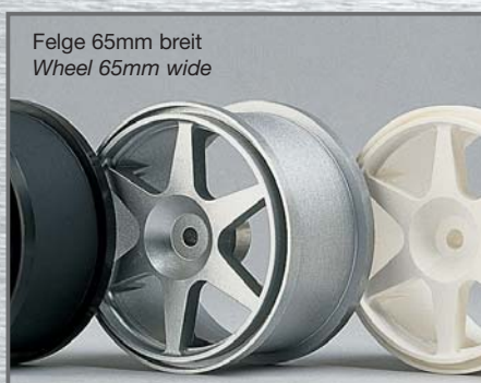
Spurverbreiternde Felge 65mm breit Track widening wheel 65mm wide
